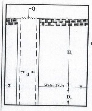
$$K = \frac{4Q}{\pi d(2H_2^2 + 4H_2D_3 + H_2d)}$$
